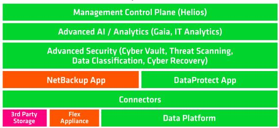
The management control plane (Helios) governs both NetBackup and DataProtect. Further, you can see that data insights modules can draw from data stored in both places. Finally, advanced security capabilities can be used with the data protection apps to provide a robust cyber resilience strategy.
